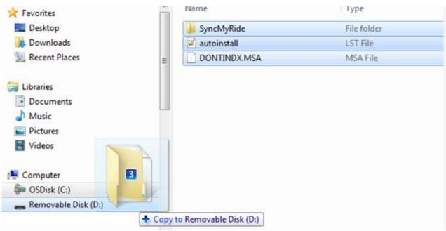
**NOTE:** Installing the software update files in your vehicle works only if the SyncMyRide folder and additional file(s)\* are visible on the USB drive. Don't combine or delete any of the files.
